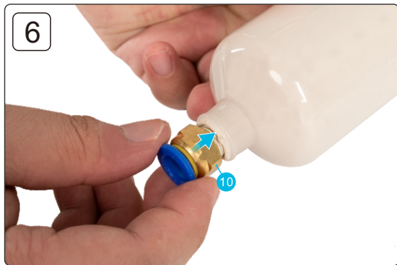
Install pc10-02 pneumatic joint on the barrel 安装PC10-02气动接头在料筒上
